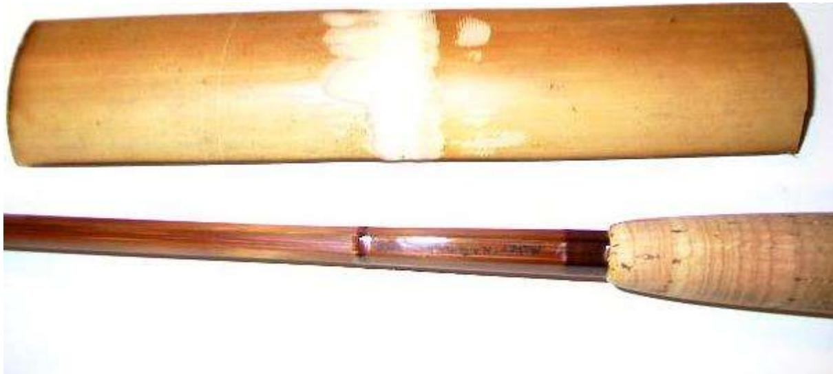
*Detail of rod with original bamboo (joint has been planed down).*
