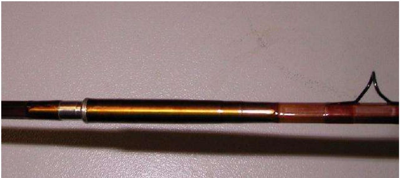
*Detail of workmanship at the ferrule - edge turned down to reduce rigidity.*
