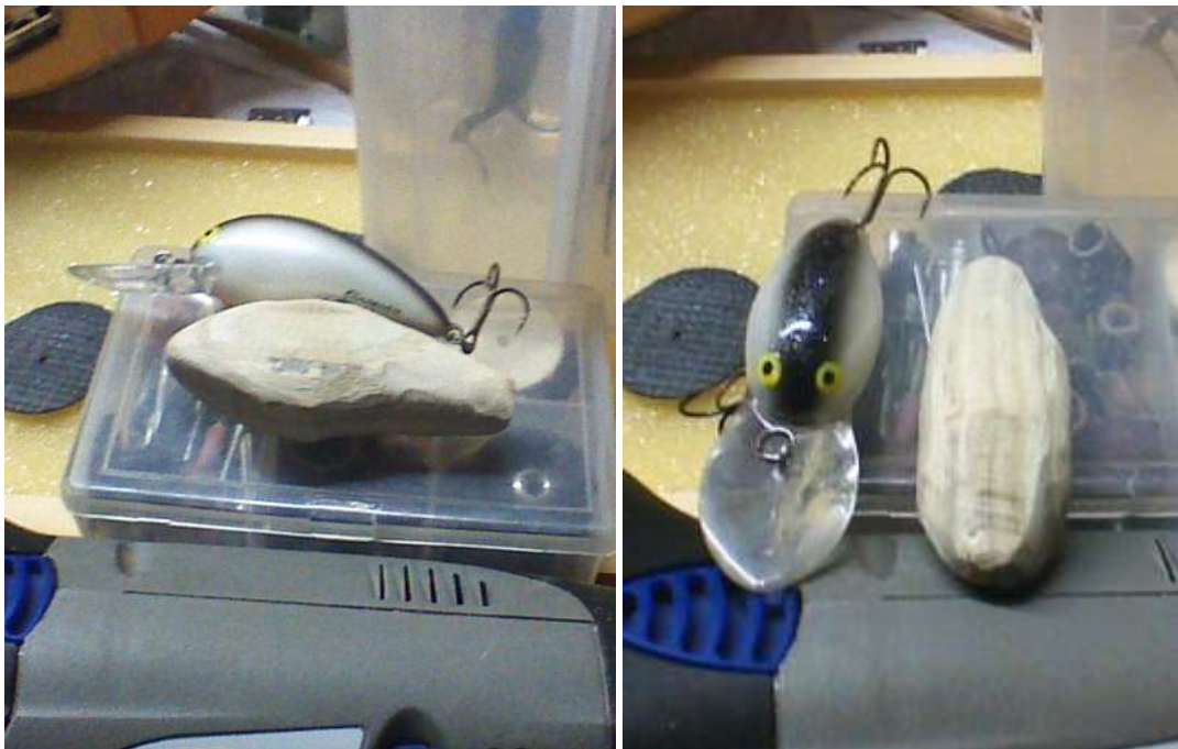
Check the shape both on the side and in profile. Try to balance it as much as possible to make the lure swimming straight, so it doesn't want to spiral or swim on its side – unless you're trying to make an injured fish, rather than a swimming lure.
