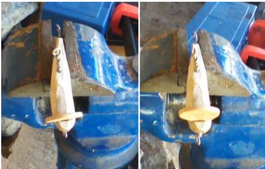
Checking the bib before gluing shows if the bib is out of alignment. It can be fixed by widening one side to straighten it, and be sure to check it whilst drying.
