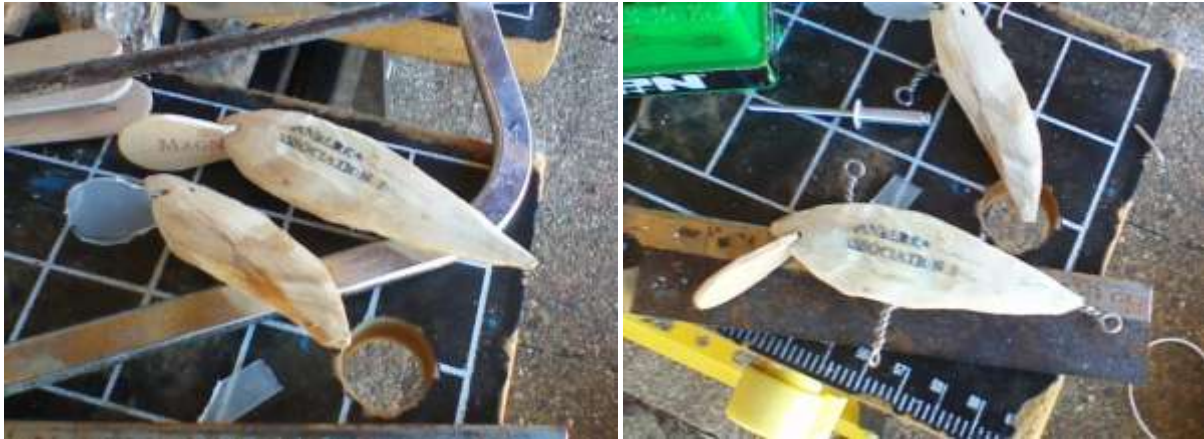
The bibs have a slight taper on the tongues. Also shown are the anchors prior to gluing.
