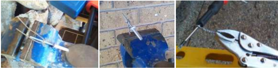
The anchors can be twisted out of wire, in a vice or pliers. Try to keep the tension even.
