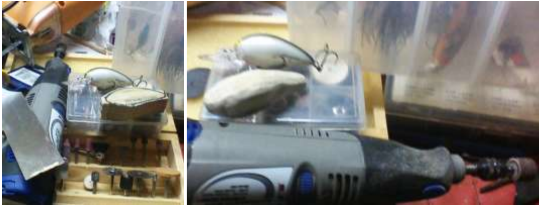
Shaping can be done with a rotary tool and a sanding attachment
