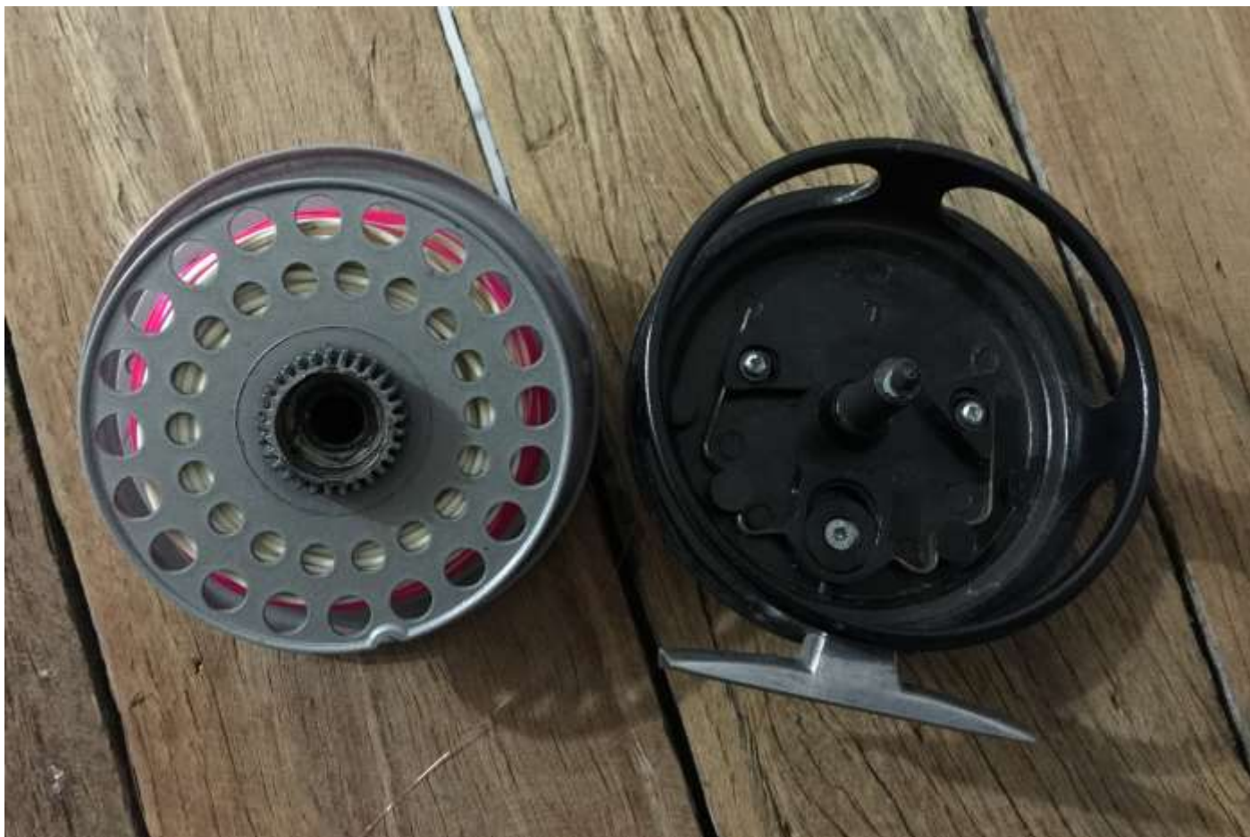
Typical 'traditional' small arbor reel. You can also see the 'clicker drag'
