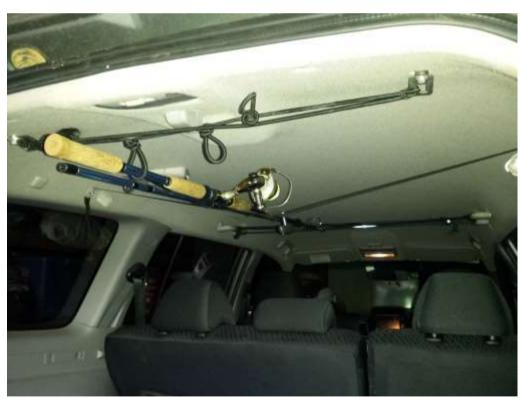
The rods are suspended against the cabin ceiling. The first problem was how to actually mount the structure. In the end I used existing hardpoints in the ceiling. There are three lines of 'straps'. The rearmost line is attached to the rear child seat brackets. The loops in the bungie cord hold the butts of the rods – the second bungie line stretches over reels when they are closer to butt.
