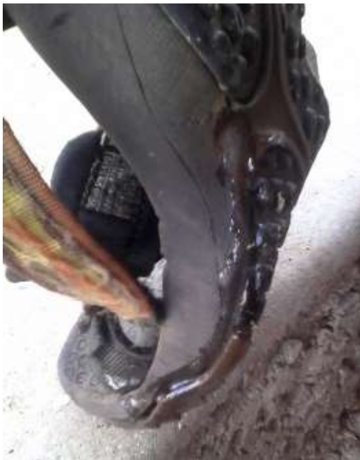
Flex test of the first shoe and the glue held up.
