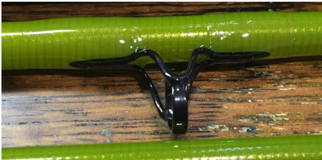
Figure 3 clear wraps under preliminary coat – final topcoat smooths out the visible dimples and rough patches
